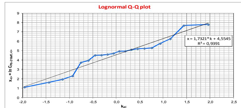
Results of Data analysis for Pb-210eff of a random sample of size n = 10 and n = 20 drawn from a population of oil sludge
